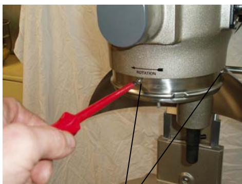
DRIP CUP & SPLASH SHIELD FIXING SCREWS (x3)
